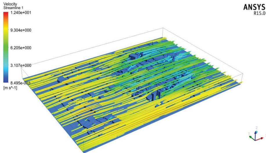
Fig. 9. Wind flow lines around the facility.
