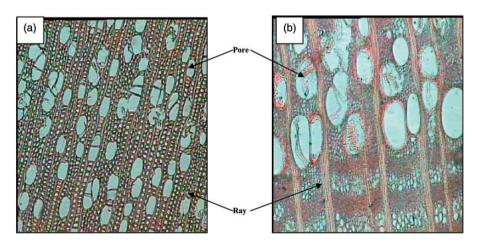
Figure 1. Cross sections of the used (a) alder (diffuse-porous) and (b) ironwood (ring-porous), magnification  $\times$  40.
