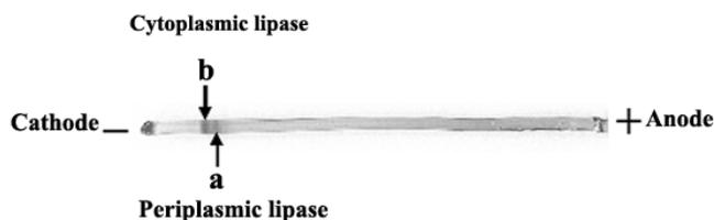
**Figure 4.** Tube capillary isoelectric focusing analysis of the purified recombinant lipase. A: cytoplasmic recombinant lipase with the signal peptide (pI of 6.50). B: periplasmic recombinant lipase without the signal peptide (pI of 6.37).
